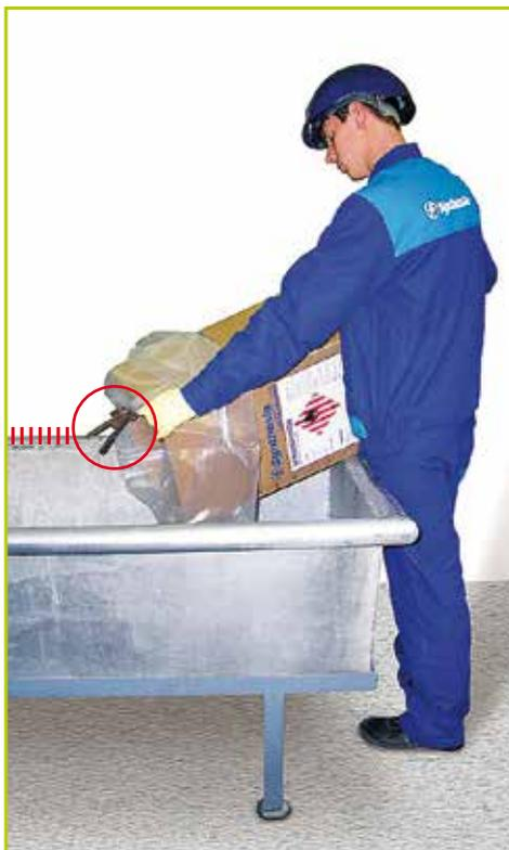
Earthing by means of an earth clip in the case of cardboard boxes (Picture 1)
